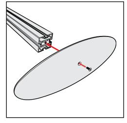
**Base Plate & Extrusion Connection**
