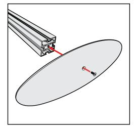
**Base Plate & Extrusion Connection**
