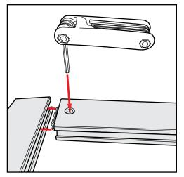
**Extrusion & Lock Connection**
